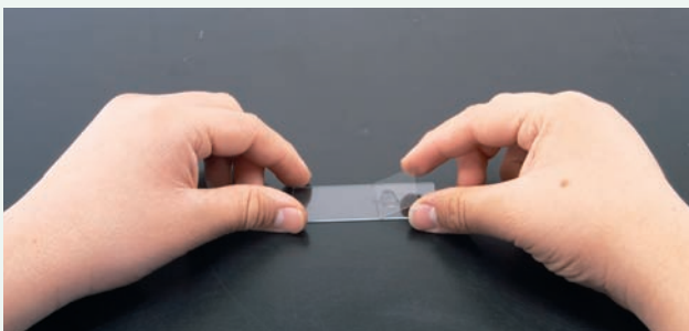
Hold the cover slip at a 45° angle and gently lower it onto the slide. There should be no air bubbles under the cover slip. If there is any excess water on the slide, dab a piece of tissue paper on the slide.
