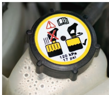
Figure 7.3B As the coolant in a car becomes hotter, it expands. The plastic container shown above provides extra space for the hot coolant to seep into. When the engine is cool, the coolant contracts and no longer overflows into the container.
