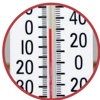
Figure 7.3A A thermometer indicates temperature through the expansion and contraction of a liquid. Because of the narrow tube, the liquid has to expand only slightly to show a large change on the temperature scale.
