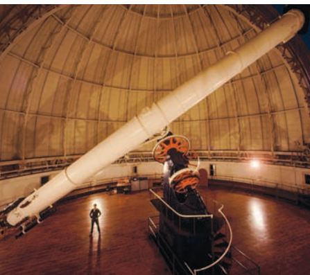
Figure 6.17 The 102 cm refracting telescope at the Yerkes Observatory in Wisconsin is the largest refracting telescope ever used.
