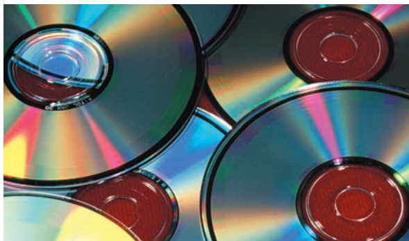
Figure 4.18 When light waves reflect from the ridges on a CD, the light waves can add together to make some colours brighter. Light waves can also cancel each other, removing some colours.
