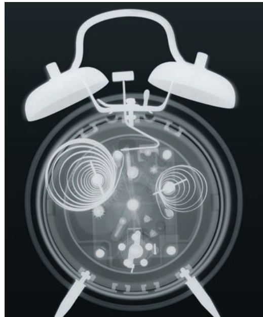
Figure 4.33 An X-ray photograph of a clock
